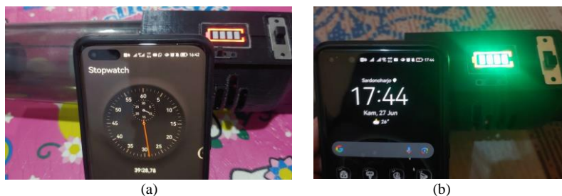
Gambar 10. Hasil pengujian charging baterai vacuum (a) status baterai saat mulai charging , (b) status baterai saat selesai charging
